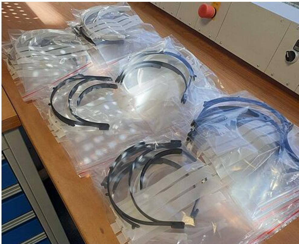
Figure 4 Hundreds of 3D-printed face-shield frames ready for assembly during the COVID-19 response. Organizations like ESA helped coordinate distributed printing efforts. (Source: ESA.)
