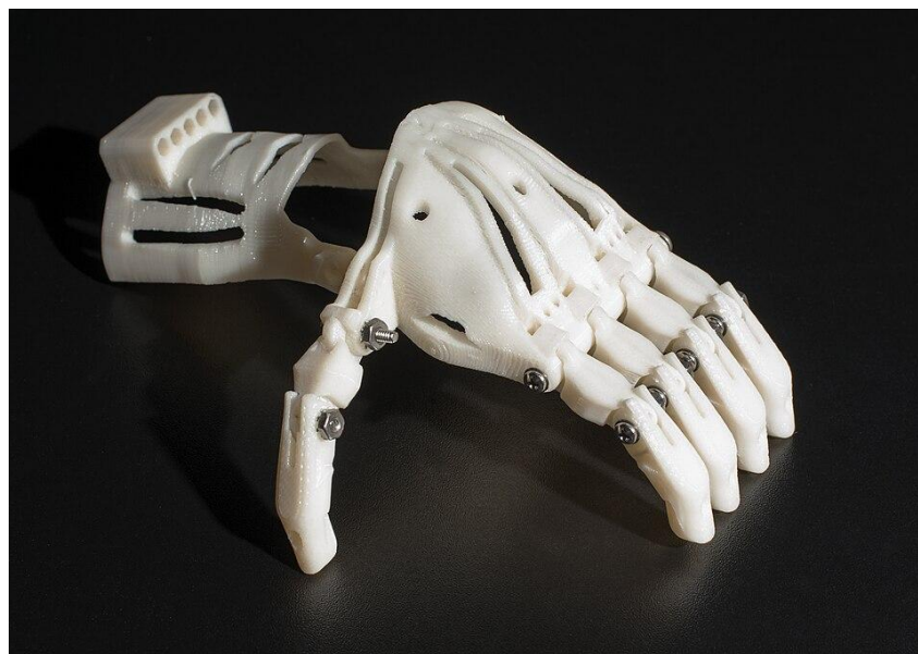
Figure 2 A 3D-printed prosthetic hand developed by FDA researchers. Such devices can be customized for patients and are much cheaper than traditional prostheses. (Source: U.S. FDA.)
